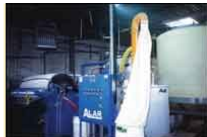
The rotary vacuum filter, left, is part of Recycle Technologies' prestripping process and uses diatomaceous earth as the filtering medium.
